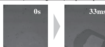
Figure 2. Optical microscopic observations of Cassie-Baxter to Wenzel wetting transition on the patterned CYTOP surfaces.
